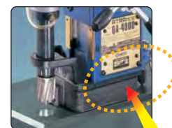
Built-in acceleration sensor inside
